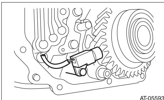
9) Remove the front vehicle speed sensor through the hole of AT transmission main case.
