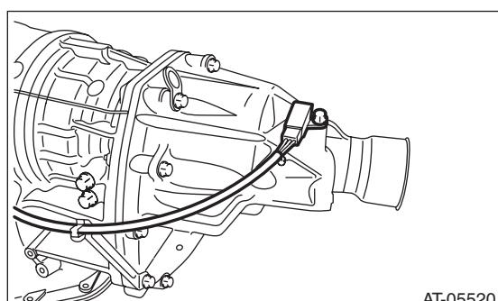
8) Install the transmission assembly to the vehicle. <Ref. to 5AT-41, INSTALLATION, Automatic Transmission Assembly.>
