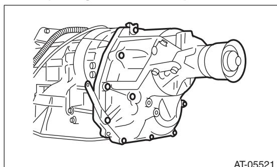
7) Connect the rear vehicle speed sensor connector.
