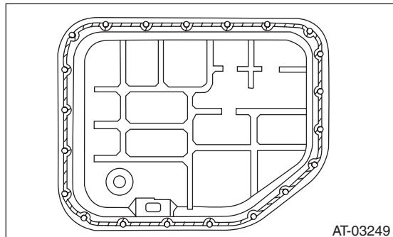
4) Install the oil pan by equally tightening the bolts.
