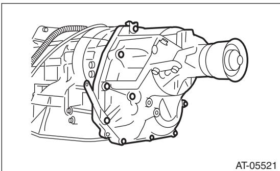
4) Remove the center differential carrier. <Ref. to 5AT-72, REMOVAL, Center Differential Carrier.>
