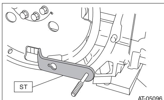
3) Tighten the drive plate mounting bolt.
