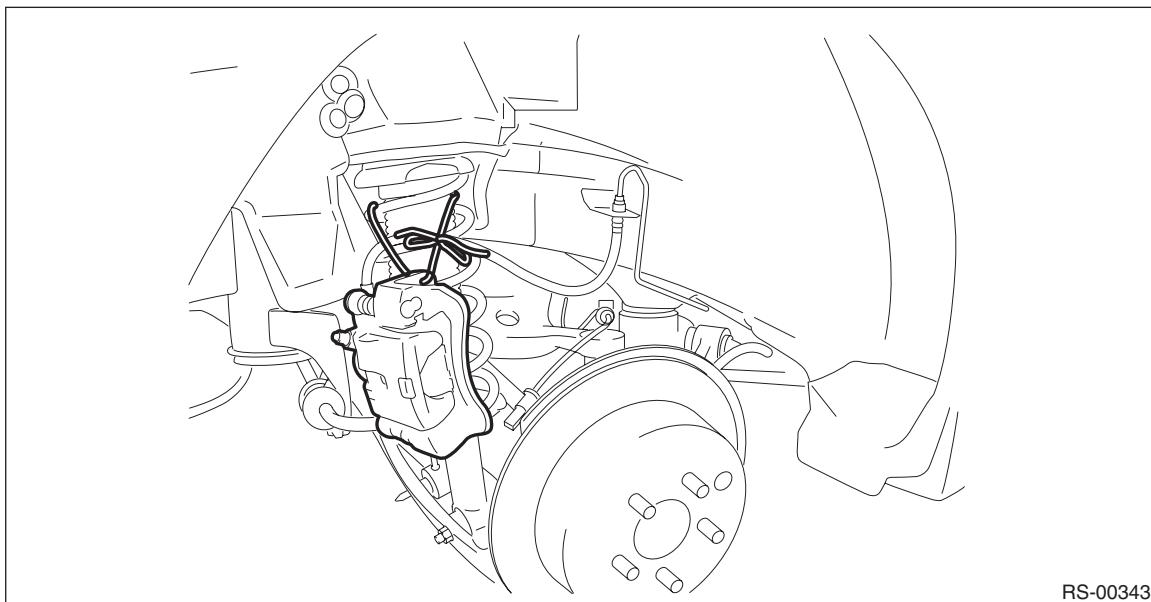
4) Remove the rear disc rotor.
