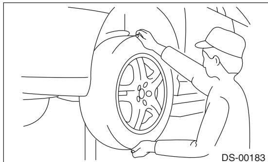
2) Inspect the lean of axis direction using a dial gauge. Replace the bearing if the load range exceeds the limitation.
