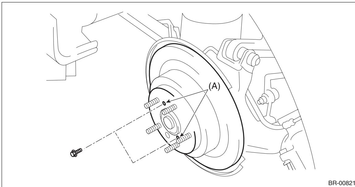
5) Remove the rear hub unit bearing.
