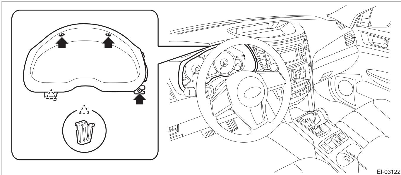
6) Remove the combination meter assembly.
