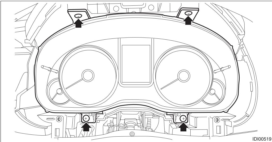
(3) Pull the combination meter toward you and disconnect the connector.
