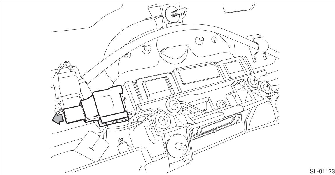
(4) Remove the screws and remove the license plate light.
