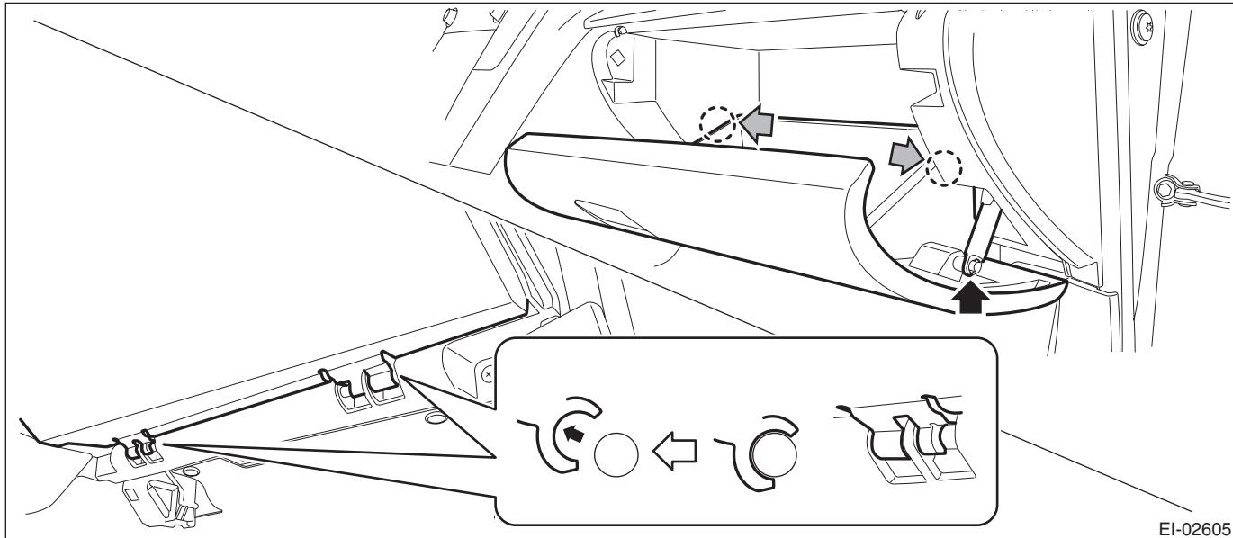
2) Release the clips, and remove the instrument panel side cover RH.
