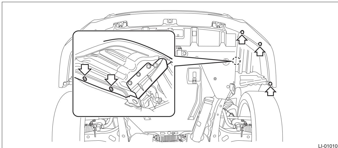
(2) Disconnect the front fog light connector. (Model with fog light)
