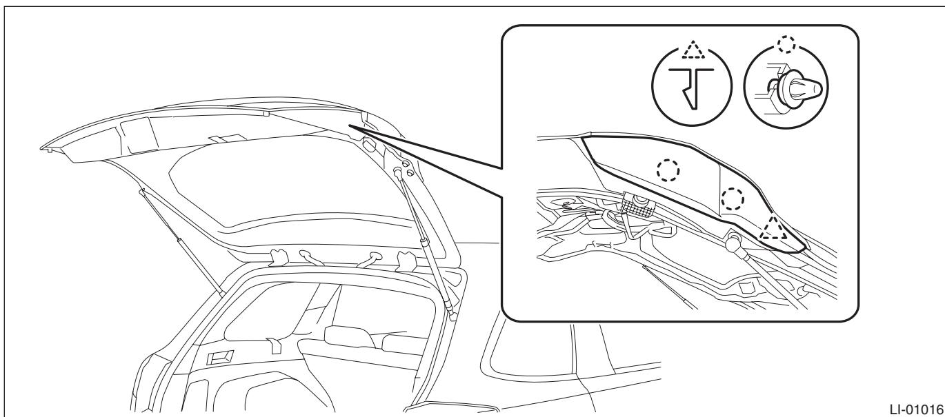
(2) Disconnect the harness connector of license plate light assembly.
