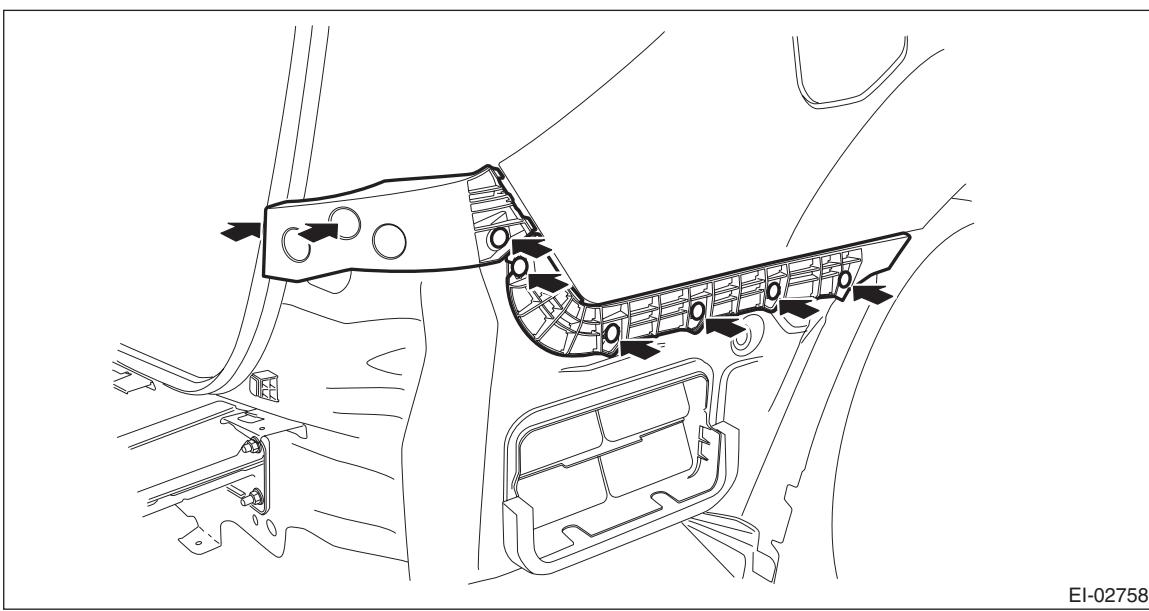
5) Remove the reflex reflector. (OUTBACK model)
