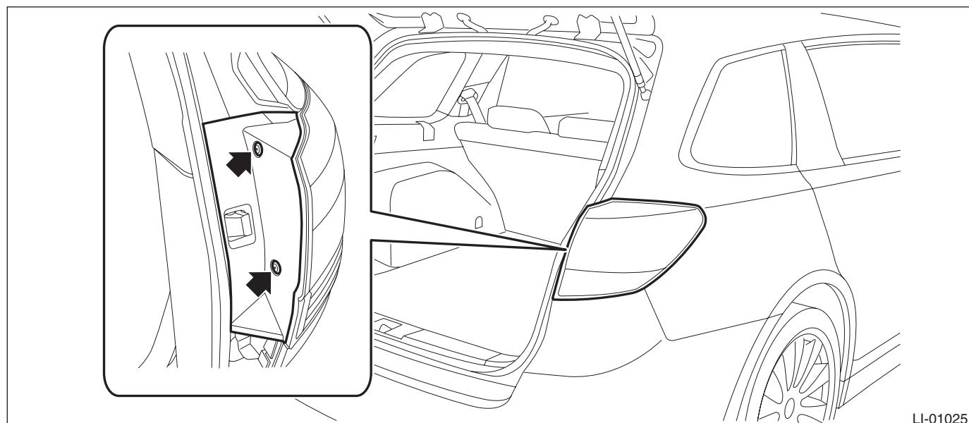
2. Release the bolts and clips, then pull out the rear combination light assembly to the vehicle rear.
