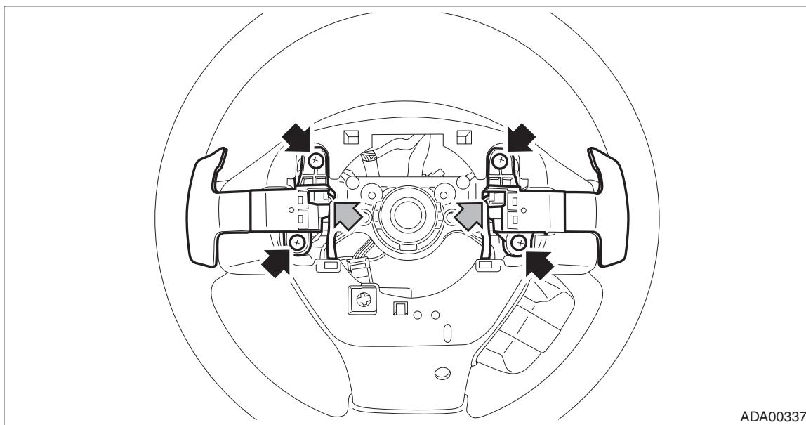
(2) Remove the steering switch connector and screw.
