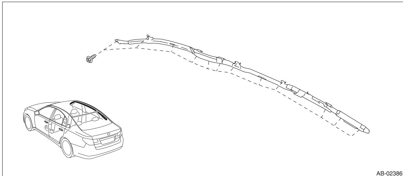
(2) Disconnect the curtain airbag module connector.
