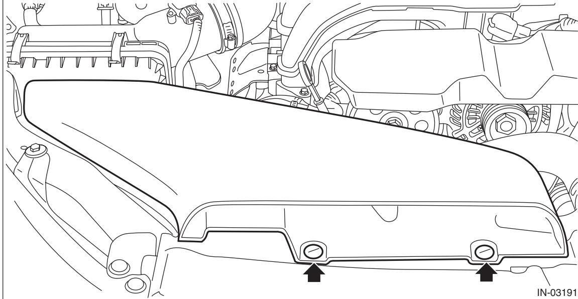
3) Turn the steering wheel in the opposite direction from the parts to be removed. Then remove the clips and turn over the mud guard.
