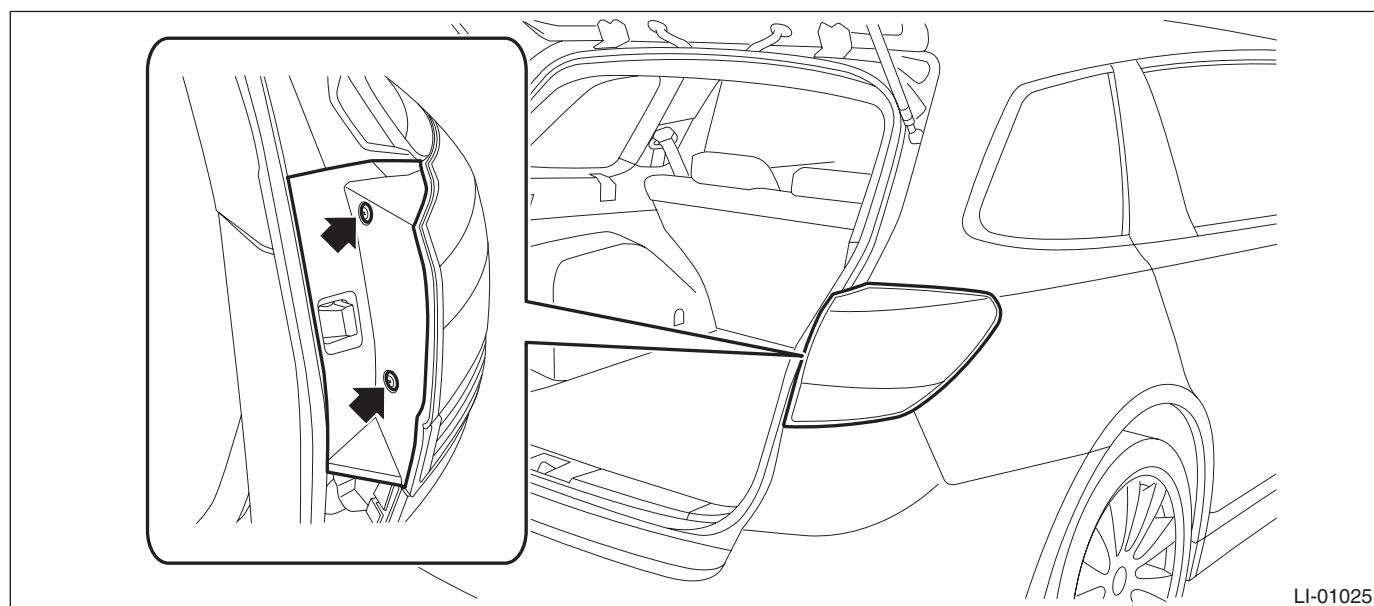
3) Remove the rear combination light assembly.
