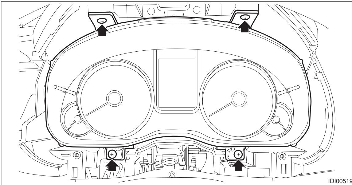
(5) Remove the combination meter assembly as shown in the figure.
