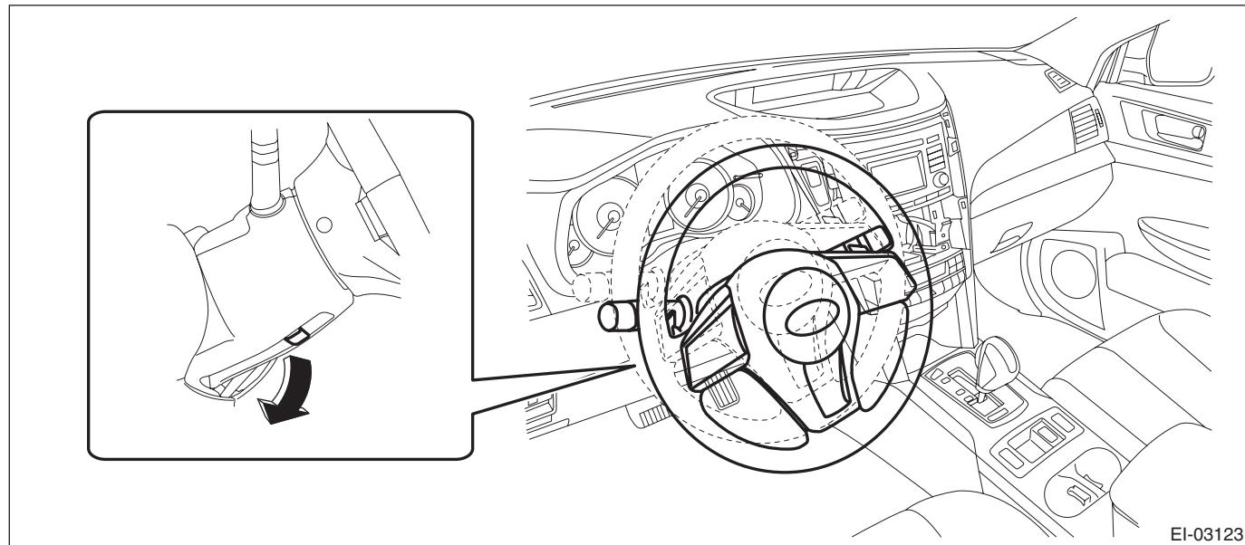
(2) Release the screws and clips, then detach the meter visor assembly.
