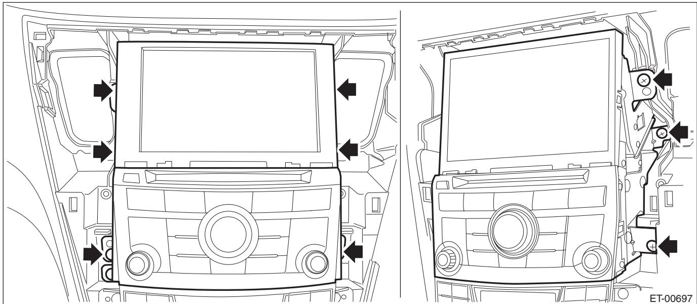
5) Remove the control panel assembly.
