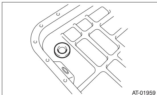
5) Apply liquid gasket to the oil pan.
