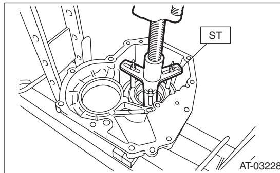
5) Install the transfer clutch. <Ref. to 5AT-66, INSTALLATION, Transfer Clutch.>
