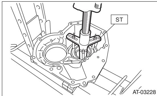
3) Supply compressed air to remove the clutch piston.
