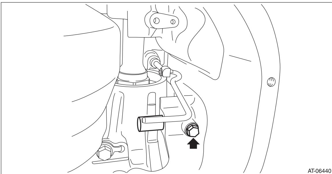
5) Install the parking rod to the manual plate.
