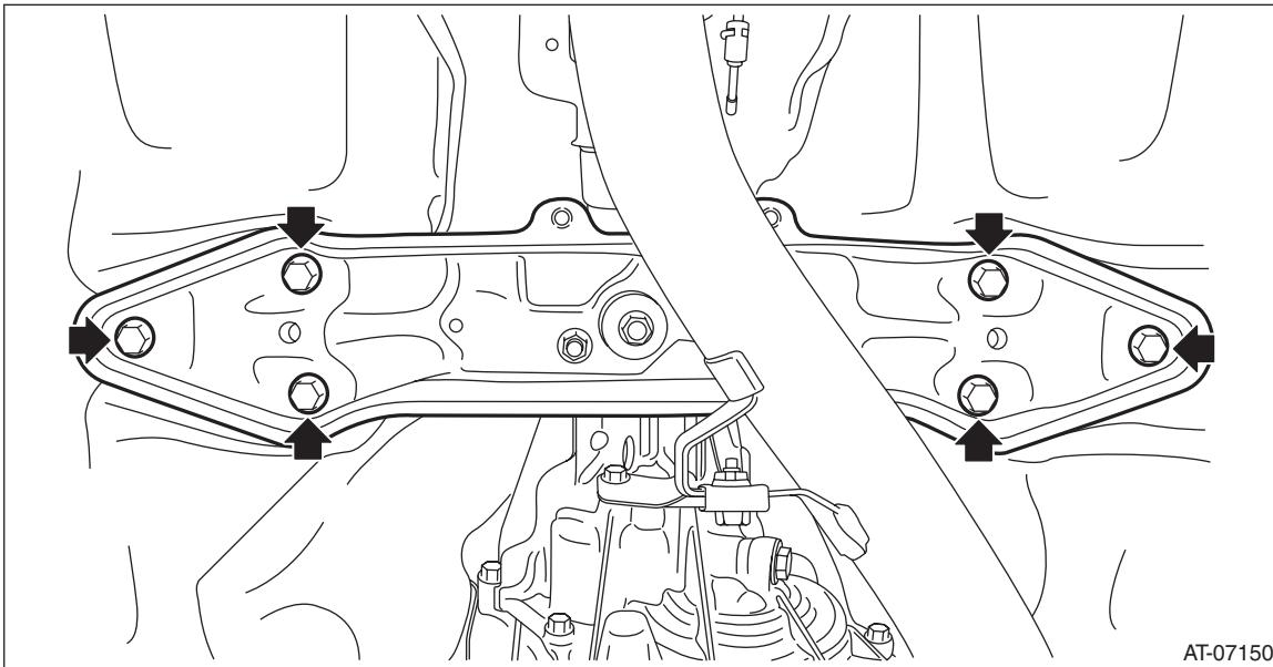
18) Lower the rear side of transmission until the ST can be removed.
