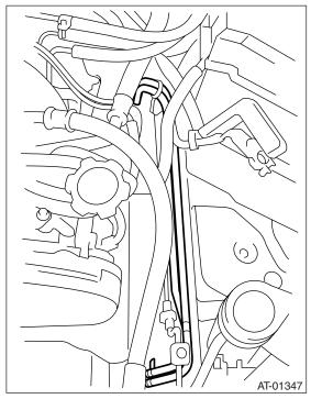
3) Attach the bolts securing the ATF cooler pipe, and attach the ATF cooler hose.
