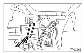
4) Attach the ATF filter inlet and outlet hoses.
