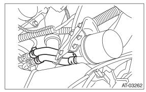
8) Remove the bolts securing the ATF cooler pipe, and remove the ATF cooler hose.
