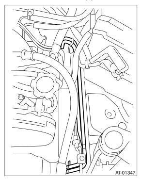
10) Remove the oil cooler inlet and outlet pipes.
