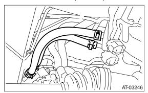
7) Connect the ATF cooler hose to the pipe on the radiator side.
