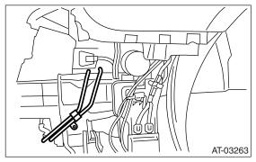
9) Disconnect the ATF cooler pipe from frame.
