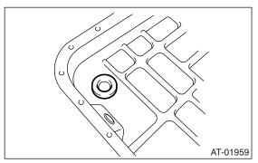
5) Apply liquid gasket to the oil pan.
