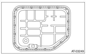
6) Install the oil pan by equally tightening the bolts.
