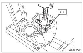
3) Supply compressed air to remove the clutch piston.
