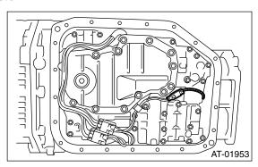
8) Remove the front vehicle speed sensor securing bolt
