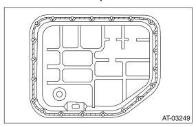
4) Install the oil pan by equally tightening the bolts.
