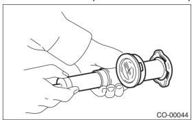
3) Increase pressure until the radiator cap tester gauge needle stops. Radiator cap is functioning properly if it holds the service limit pressure for 5 — 6 seconds. Replace the radiator cap if its valve opens at less than the service limit.
