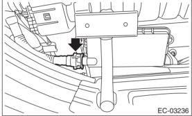
4) Remove the drain filter from the vehicle.
