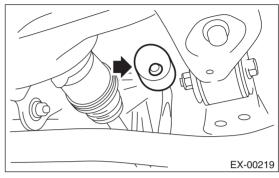
6) Remove the rear exhaust pipe.
