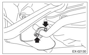
4) Apply a coat of spray type lubricant to the mating area of cushion rubber.
