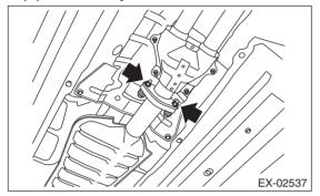
3) Remove the rear exhaust pipe from the muffler.
