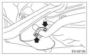
4) Install the rear exhaust pipe to the front exhaust pipe assembly.
