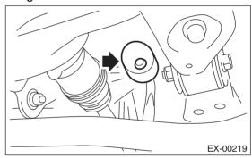
3) Install the rear exhaust pipe to the muffler.
