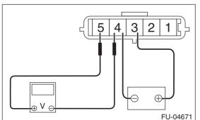
2) Check the voltage changes when air is blown to the mass air flow sensor unit in arrow direction.
