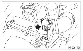
3) Remove the mass air flow and intake air temperature sensor.
