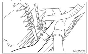
3) Disconnect the connectors from the mass air flow and intake air temperature sensor.
