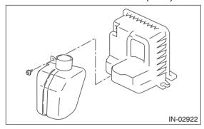
2) Separate the resonator chamber and the air cleaner case (front).
