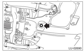
4) Tighten the engine oil drain plug after draining engine oil.
