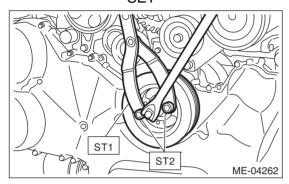
3) Remove the crank pulley.
