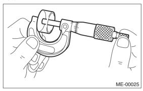
6) Select a valve lifter of suitable thickness using the measured valve clearance and valve lifter thickness, and install it.
