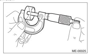
8) Select a valve lifter of suitable thickness using the measured valve clearance and valve lifter thickness, and install it.
