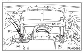
(5) Remove the air intake chamber, and move it to the left side wheel apron.
