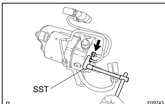
(b) Using SST, disconnect the 2 brake lines from the precharge pump.
