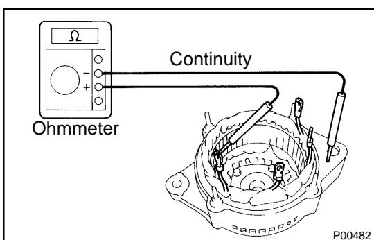
(b) Inspect the stator for ground.
