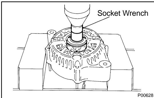
(c) Using SST and a press, press in a new bearing.
