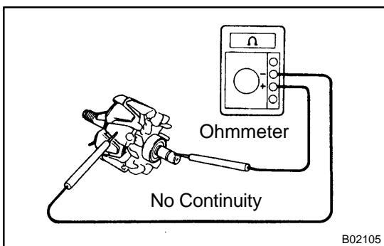
(b) Inspect the rotor for ground.
