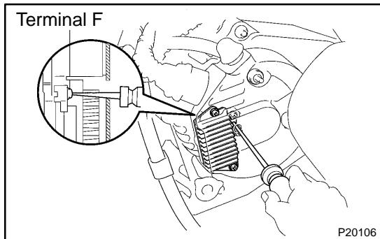
If the voltmeter reading is less than standard voltage, check the voltage regulator and generator as follows:
