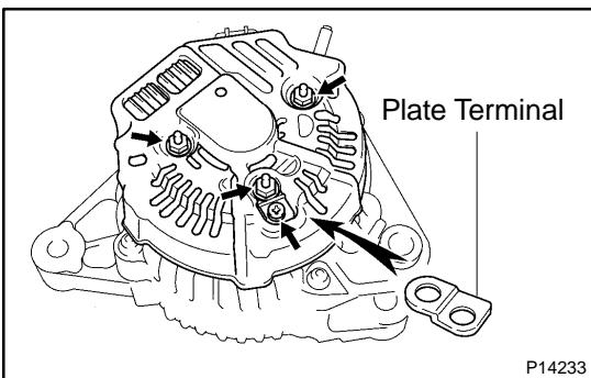
(b) Remove the screw, 3 nuts, plate terminal and end cover.
