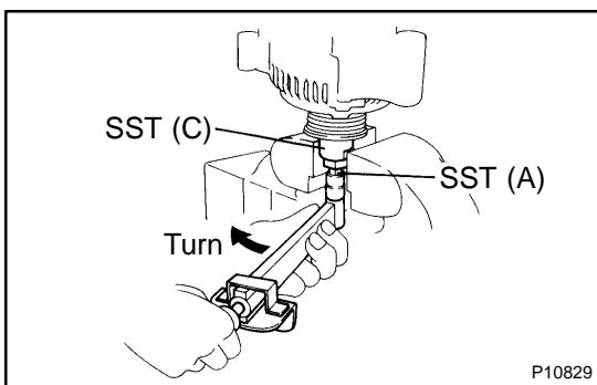
(f) To torque the pulley nut, turn SST (A) in the direction shown in the illustration.
