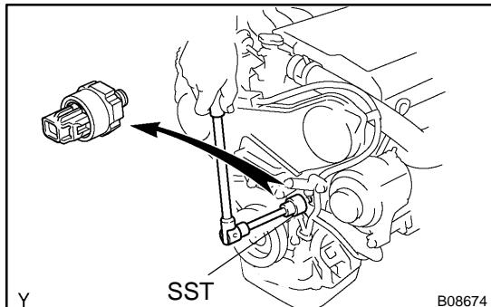
(b) Install the oil pressure gauge.
