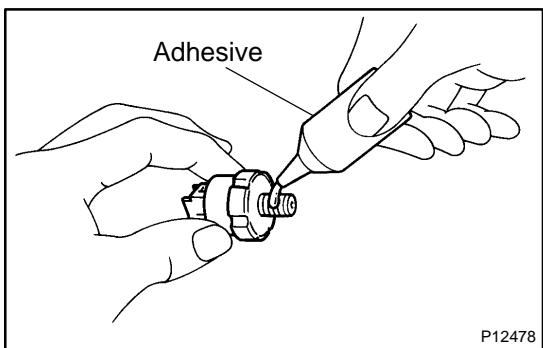
6. **REMOVE OIL PRESSURE GAUGE AND REINSTALL OIL PRESSURE SWITCH**
