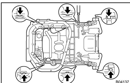
(c) Using a screwdriver, remove the oil pan by prying the portions between the cylinder block and oil pan.
