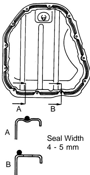
(b) Apply seal packing to the No.2 oil pan as shown in the illustration.
