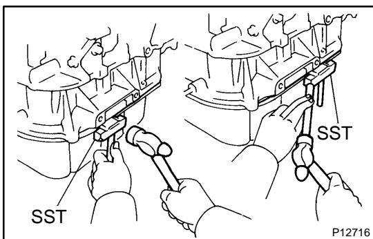
(b) Insert the blade of SST between the No.1 and No.2 oil pans, and cut off applied sealer and remove the No.1 oil pan.
