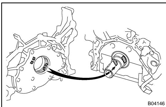
(d) Engage the spline teeth of the oil pump drive gear with the large teeth of the crankshaft, and slide the oil pump on the crankshaft.
