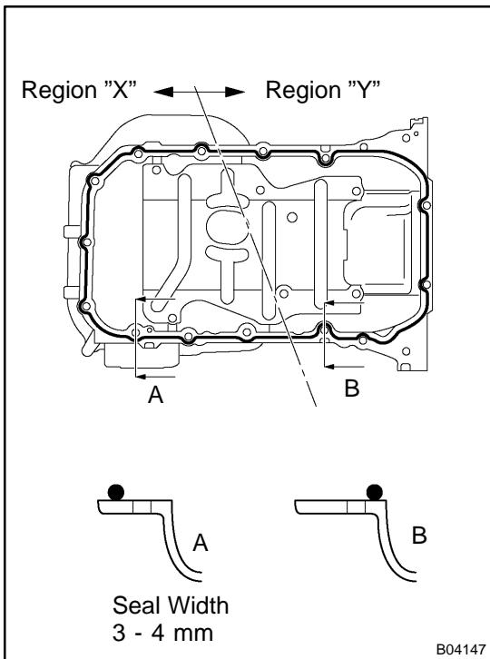
(b) Apply seal packing to the oil pan as shown in the illustration.
