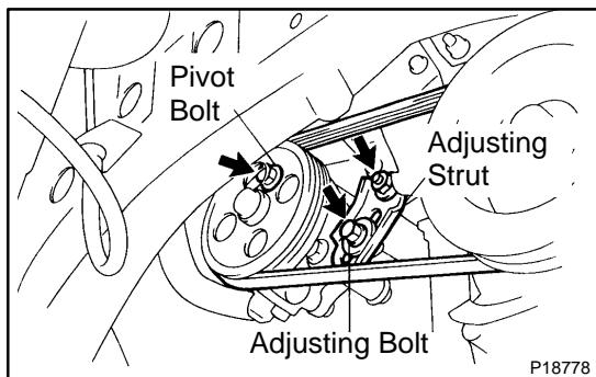
7. REMOVE PS PUMP DRIVE BELT AND ADJUSTING STRUT
