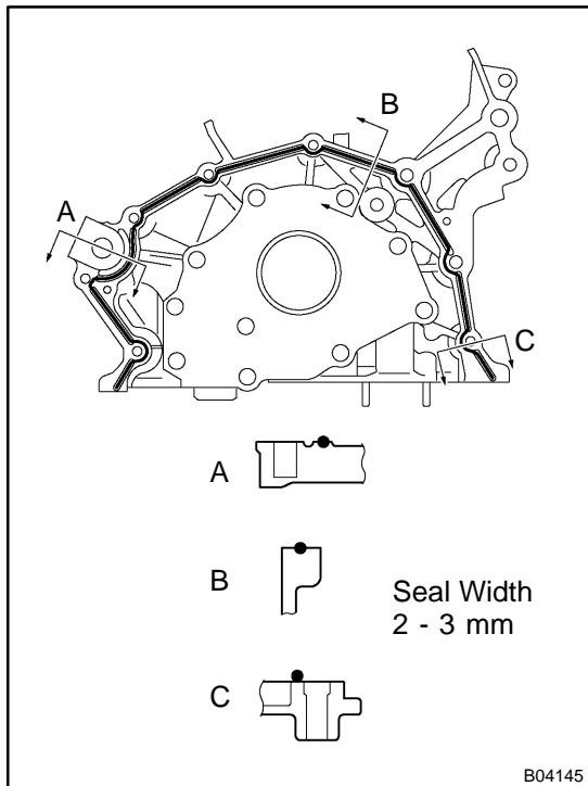
(b) Apply seal packing to the oil pump as shown in the illustration.
