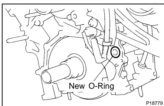
(c) Place a new O-ring on the cylinder block.
