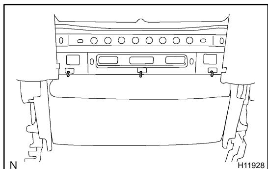
(b) Install 3 new hog rings as shown in the illustration.
