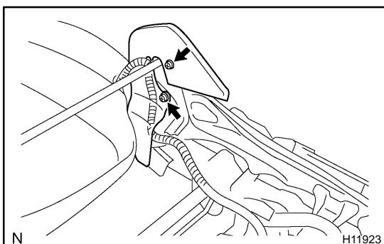
(c) Remove the 2 screws and reclining adjuster inside cover.
