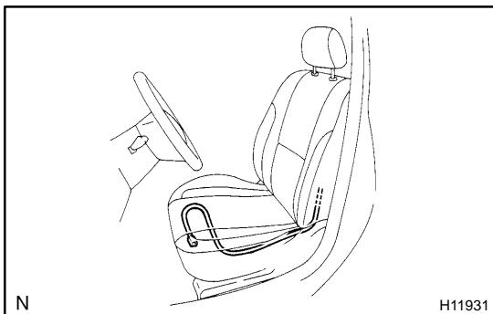
(b) Disconnect the side airbag connector.
