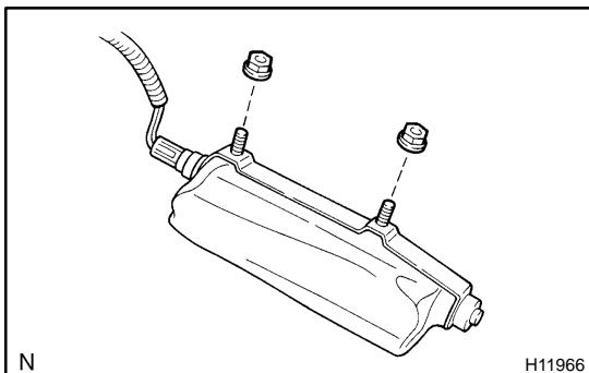
(1) Install the 2 nuts to the side airbag assembly.
