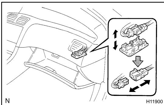
(b) Disconnect the airbag connector.
