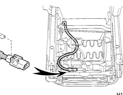
(c) Install the wire harness to the seat cushion assembly.
