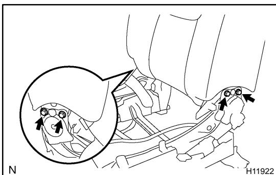
(b) Remove the 4 bolts and seatback assembly.
