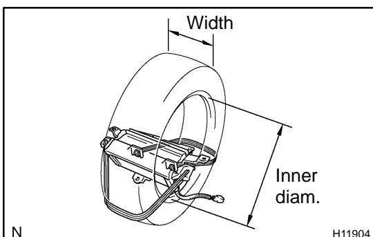
(2) Position the front passenger airbag assembly inside the tire with the airbag deployment side facing inside.
