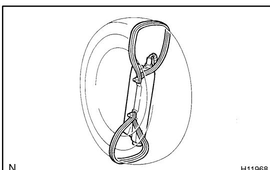
(3) Position the side airbag assembly inside the tire with the airbag deployment direction facing inside.
