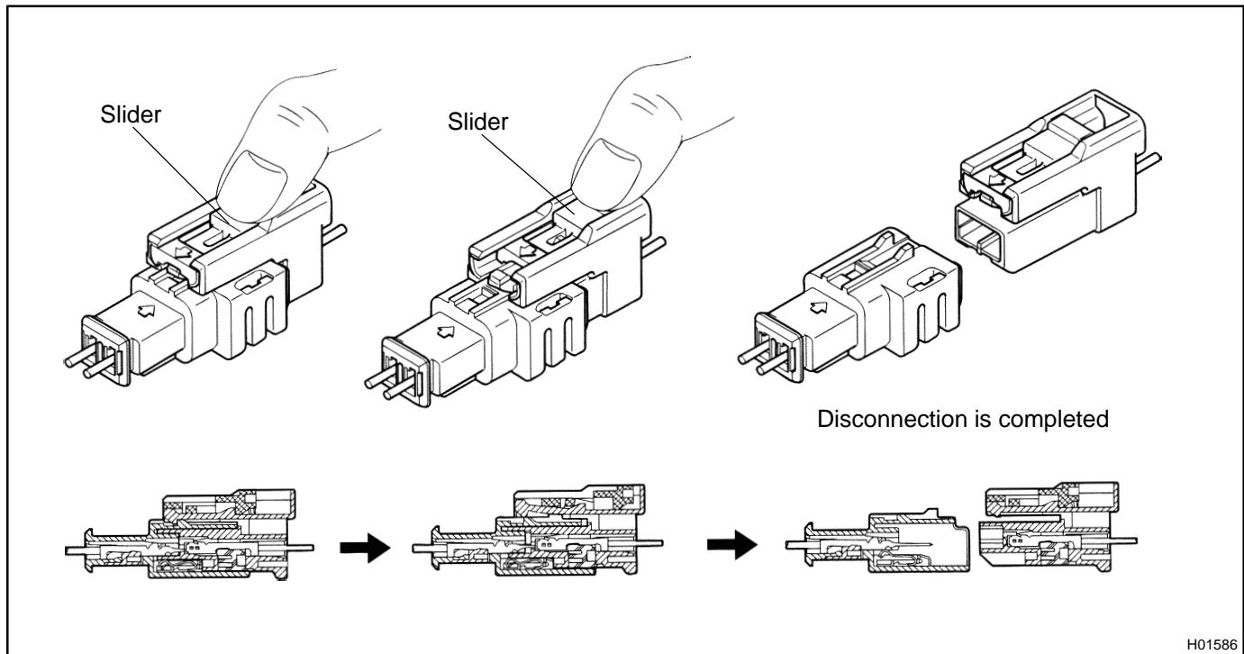
**16. CONNECTION OF CONNECTORS FOR STEERING WHEEL PAD (with AIRBAG) AND FRONT PASSENGER AIRBAG ASSEMBLY**
