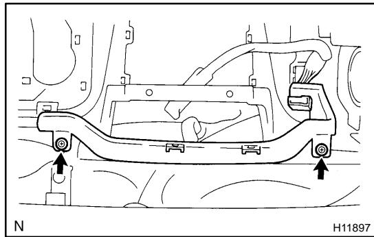
(c) Remove the 2 screws and part of instrument panel wire harness, as shown in the illustration.
