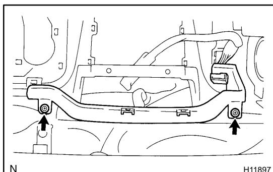
(c) Install part of the instrument panel wire harness with the 2 screws.
