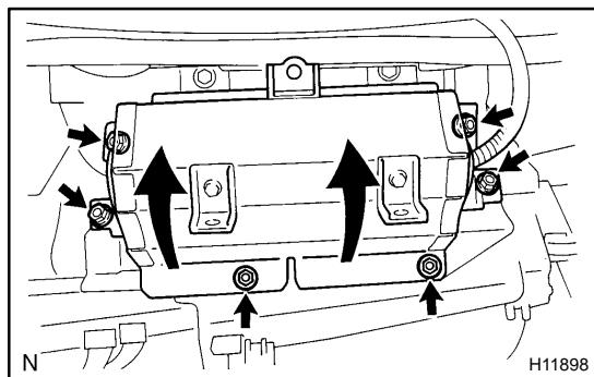
(e) Remove the 6 nuts and front passenger airbag assembly, as shown in the illustration.
