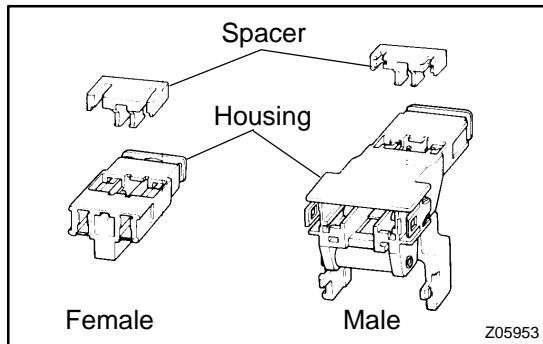
(1) Terminal Twin-Lock Mechanism
