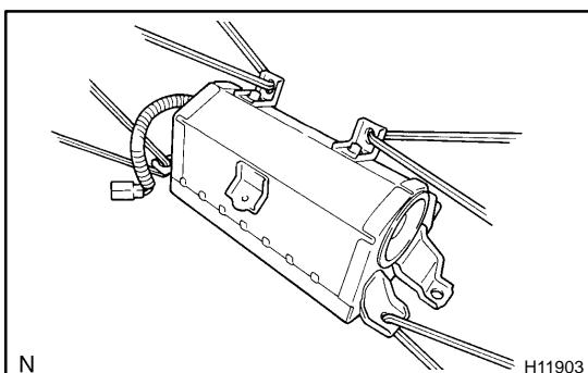
(1) Pass the wire harness though the installation holes, as shown in the illustration.
