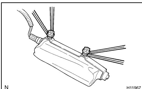
(2) Wind the wire harness around the stud bolts of the side airbag assembly as shown in the illustration.
