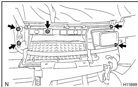
(b) Install the No. 1 safety pad with the 5 screws.
