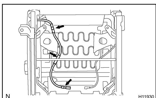
(c) Install the wire harness of the side airbag assembly to the seat cushion assembly.
