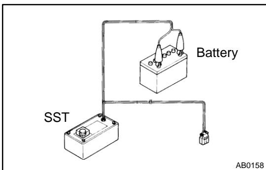
(c) Check functioning of the SST (See step 1-(a) on page [RS-17](#) ).
