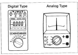
(c) Use a volt/ohmmeter with high impedance (10 kΩ/V minimum) for troubleshooting of the electrical circuit.
