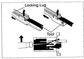
(c) Release the locking lug from terminal and pull the terminal out from rear.
