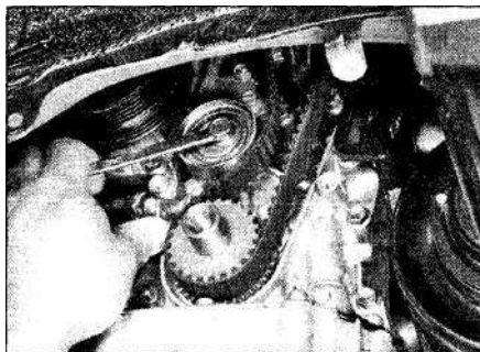
5.12a Retighten the bolt to keep the tension off the belt for removal/installation
