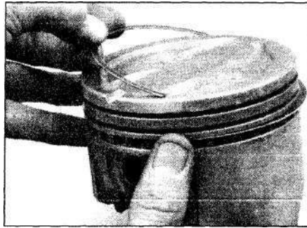
19.9b Do not use a piston ring installation tool when installing the oil ring side rails
