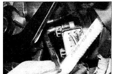
4.15 Undo the screws securing the ignition/starter switch to the rear of the lock cylinder housing
