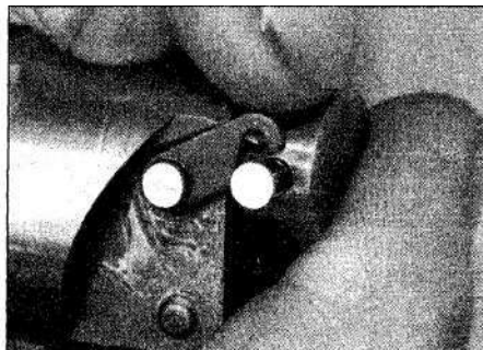
6.36b ... then retain it with the hook
