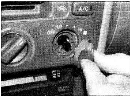
4.45a Pull the heater control knobs from place ...
