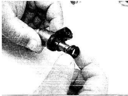
12.44b Remove the grommet from the top of the injector
