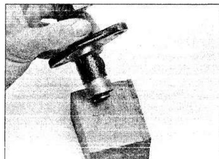
5.8 Invert the cylinder and tap it against a block of wood to eject the piston
