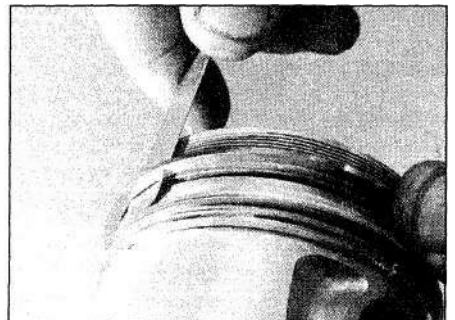
15.2 Use old feeler gauge blades to carefully expand the piston rings
