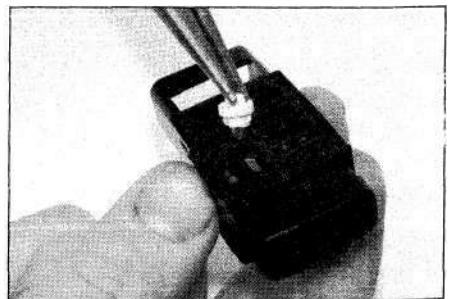
8.24 Use a pair of thin-nosed pliers to rotate the hazard light illumination bulbholder anti-clockwise
