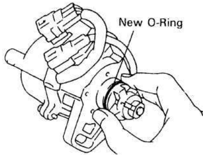
3.8 Fit a new O-ring to the distributor housing
