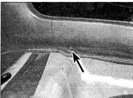
27.18 Unscrew the tailgate sill trim panel plastic nuts (right-hand nut arrowed)
