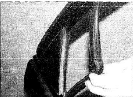
15.10 Prise out the window rubber guide from the door frame
