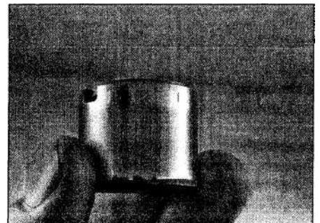
10.14 Wipe off the oil and inspect each follower for wear and scuffing
