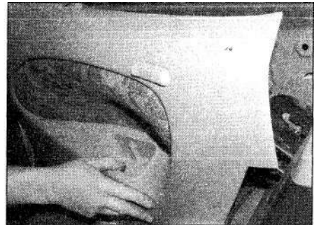
27.17b ... then pull the side panel from place
