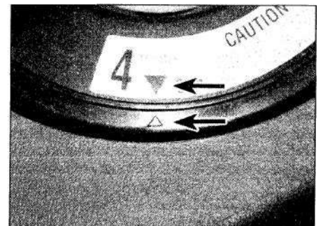
16.7 Align the contact reel pointers (arrowed)
