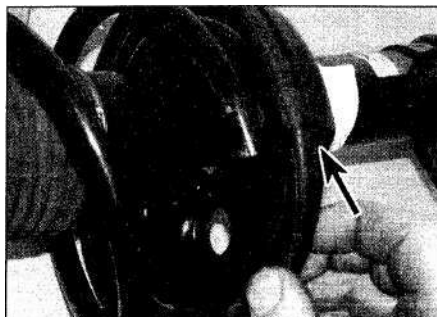
3.16 The end of the spring must rest in the lowest part of the insulator (arrowed)
