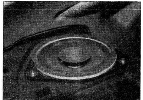
18.8 The rear speakers are retained by three screws
