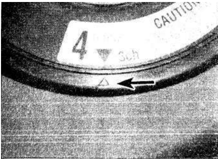
20.10 When centralised, the arrows on the contact unit should align (arrowed)
