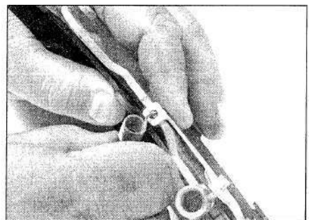
11.5q ... hook the short end of the adjusting lever spring into the shoe lever...
