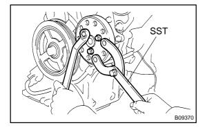
(b) Using SST, install the pump pulley with the 3 bolts. SST 09960-10010 (09962-01000, 09963-00600)
