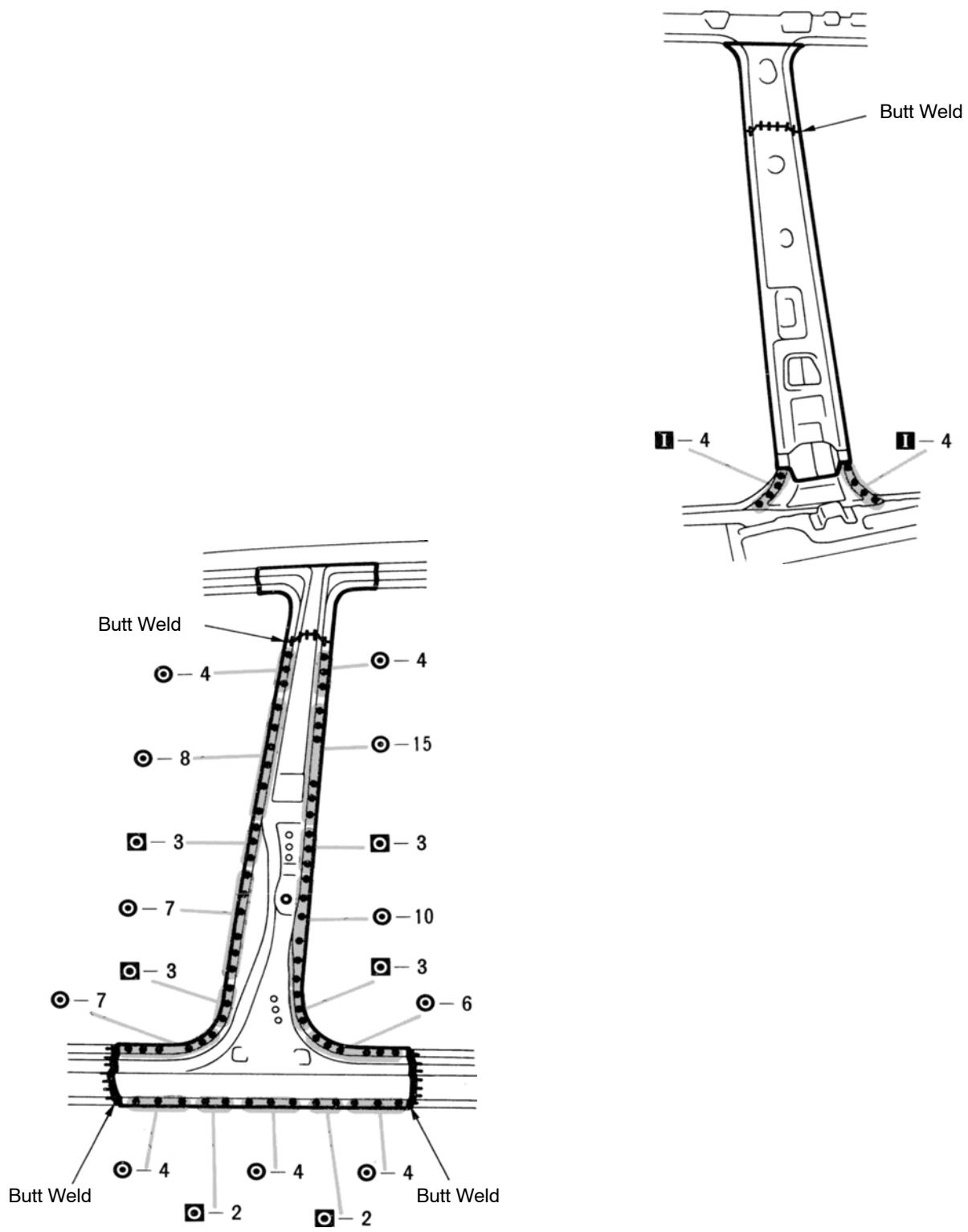
1. Temporarily install the new parts and measure each part in accordance with the body dimension diagram.
