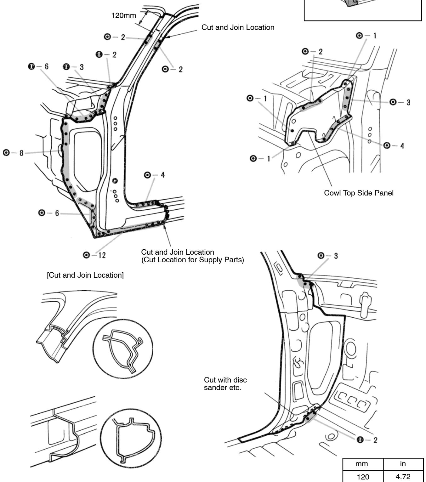
1. Cut and join the parts at the locations shown above.
