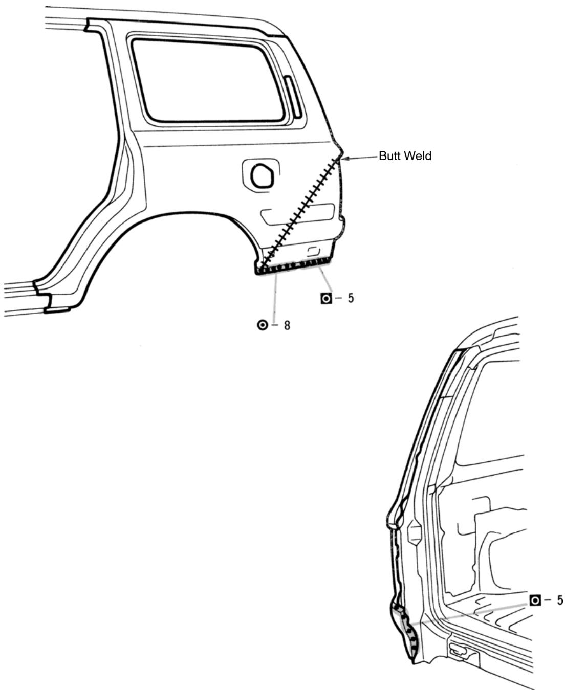
1. Temporarily install the new parts and check the fit of the back door and rear combination light.
