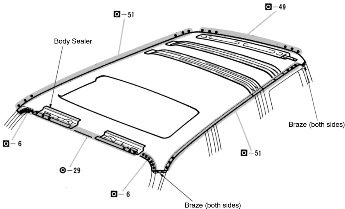
1. Before temporarily installing the new parts, apply body sealer to the windshield header panel, roof panel reinforcement and back door opening frame.
