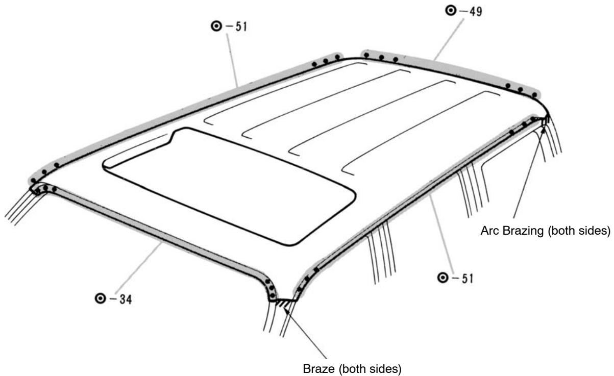
1. Heat the brazed area of the front body pillar and scrape off the brazing with a wire brush.
