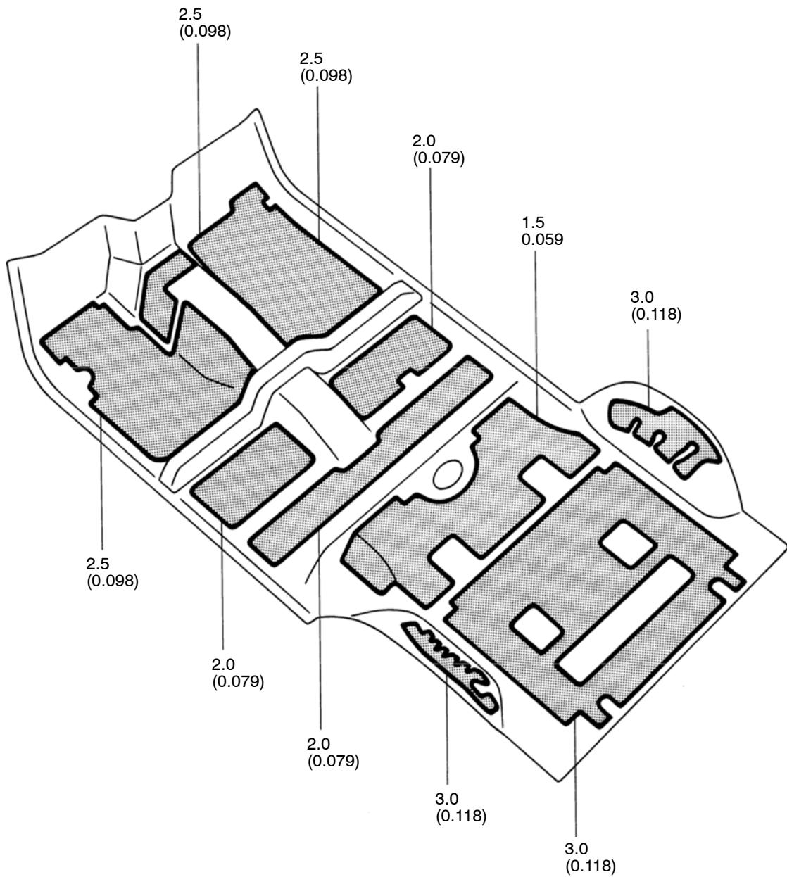
mm (in.): The numbers in the diagram indicate the thickness of the silencer sheet.
