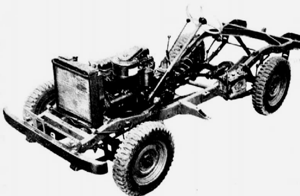
FIG. 3 MODELS BJ25 AND BJ25L CHASSIS
