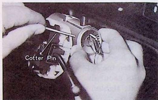
Fig. 2-21 Key Cylinder Replacement
