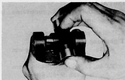
Fig. 2-57 Installing Joint Spider V5126
