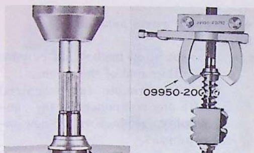
Fig. 2-40 Removing Inner Race
