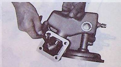
Fig. 1-10 Removing Front V5061 Drive Shift Fork
