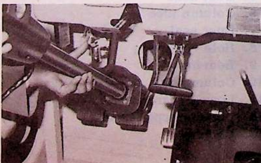
Fig. 2-5 Main Shaft Removal
