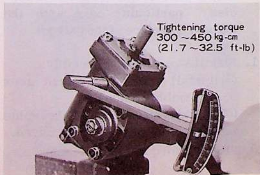
Fig. 2-50 Reinstalling Sector Shaft
