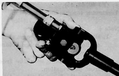
Fig. 2-58 Tightening U-bolt Nut V5127
