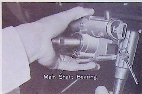
Fig. 2-10 Upper Bracket Removal
