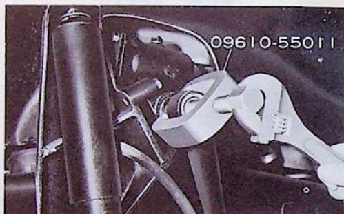
Fig. 2-25 Removing Pitman V5129 Arm
