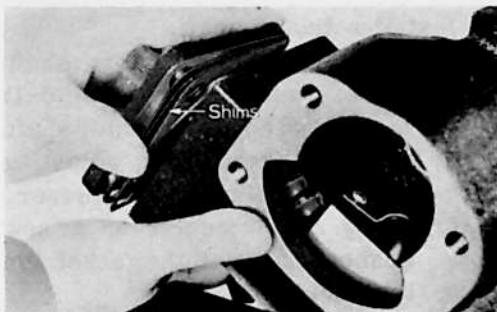
Fig. 2-46 Reinstalling Worm Gear
