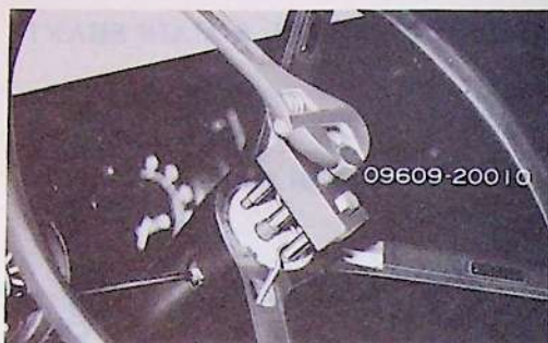
Fig. 2-2 Removing Steering Wheel V5136
