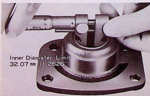
Fig. 2-35 Measuring End Cover Bushing
