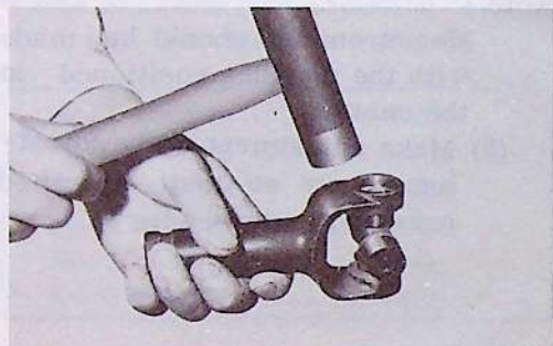
Fig. 2-55 Removing Spider V5131 Bearing
