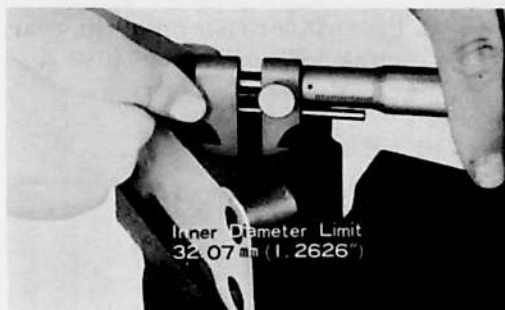
Fig. 2-37 Measuring Bushing Inner Dia.
