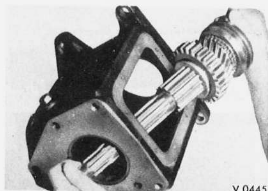
Fig. 3-21. Removing the spline shaft with attached parts through the transmission case cover hole.
