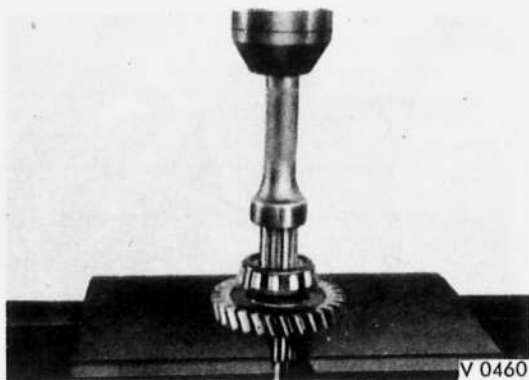
Fig. 3 36. Removing the cone of tapered roller bearing from the transfer drive shaft.
