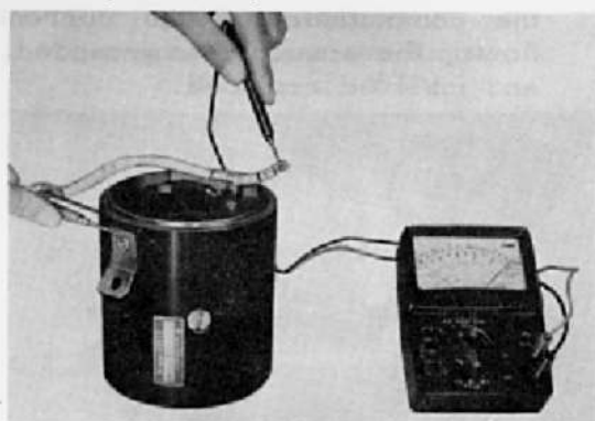
Fig.7-11 Testing Field Coil for Open Circuit W4990
