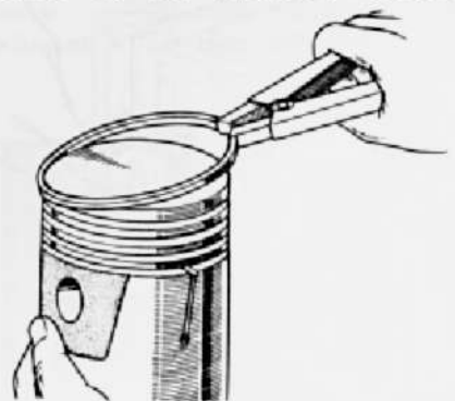
Fig. 2-6 Piston Ring Removal X4928
