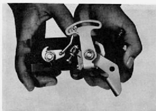
Fig. 4-53 Primary Throttle Shaft Arm Removal V0799
