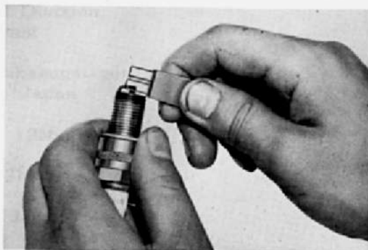
Fig.7-56 Adjusting Spark Plug Gap W0544
