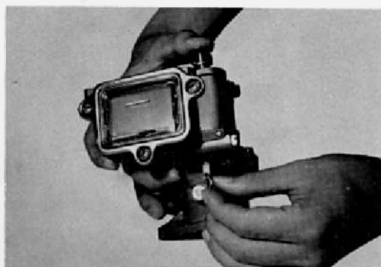
Fig.4-13 Lifter Rod Removal V0556
