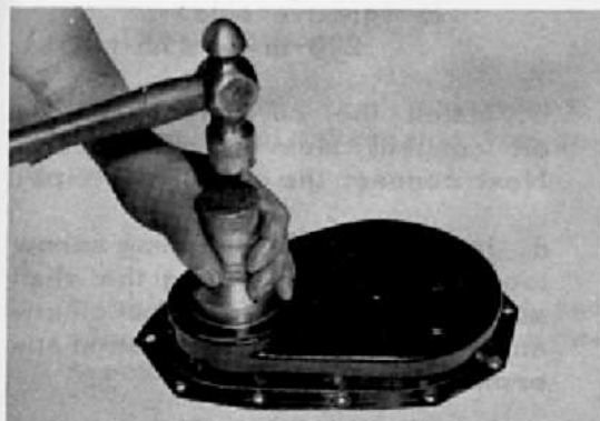
Fig.2-52 Installing Gear Cover Oil Seal V0550
