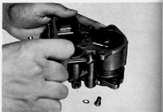
Fig.4-21 Pump Jet Removal V0564
