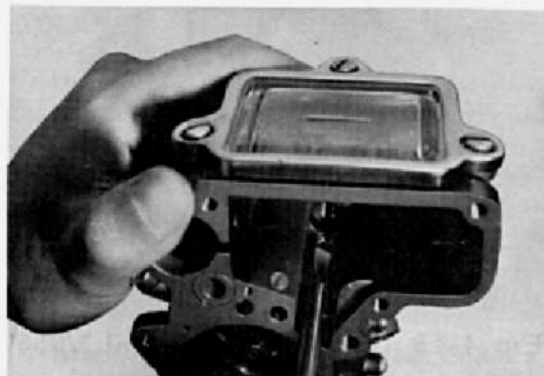
Fig.4-15 Main Jet Removal V0558
