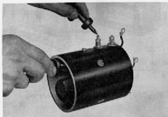
Fig.7-28 Testing Field Coil for Short W2748
