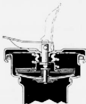
Fig.6-9 Pressure Type Radiator Cap (FA, FC) X5052
