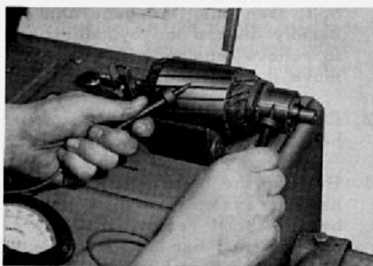
Fig.7-24 Testing Armature Commutator for Short W2744
