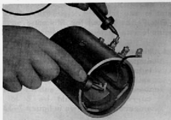
Fig.7-27 Testing Field Coil for Open Circuit W2746
