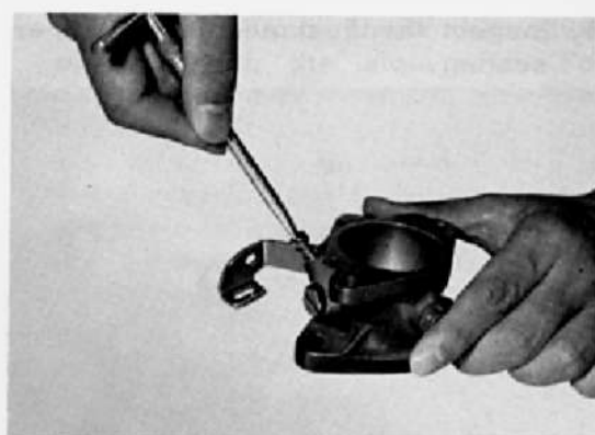
Fig.4-24 Idle Adjusting Screw Removal V0567
