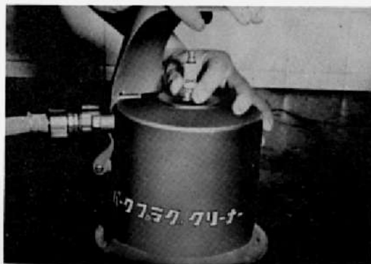
Fig.7-55 Cleaning Spark Plug W0543
