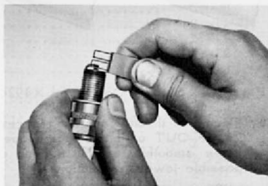
Fig.1-10 Adjusting Spark Plug Gap W0544
