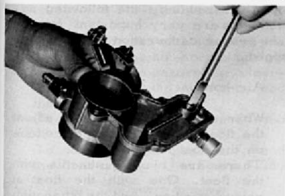
Fig.4-23 Valve Seat Removal V0566
