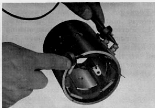
Fig.7-29 Testing Terminal for Short W2747
