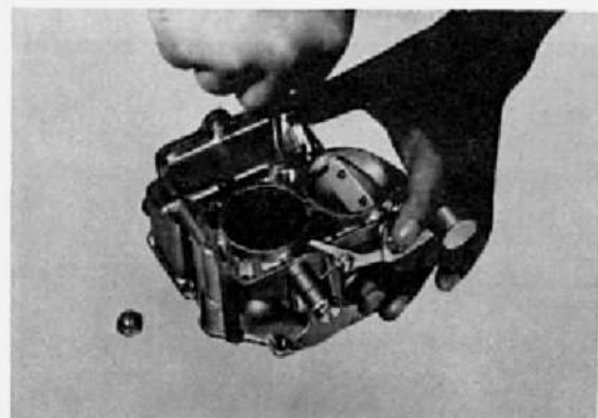
Fig. 4-52 Check Valve Removal V0798
