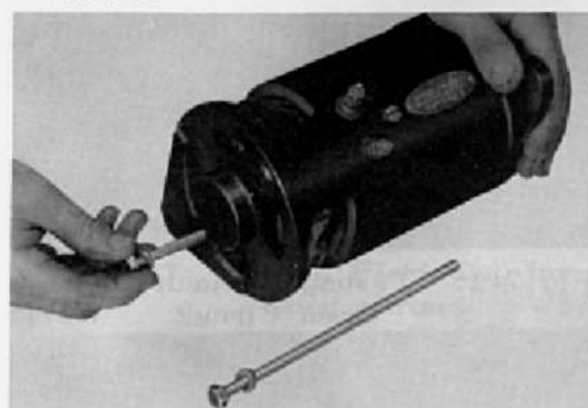
Fig.7-20 Removing Through Bolt W2740
