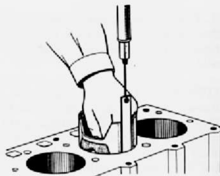
Fig.2-25 Measuring Piston Clearance X4941
