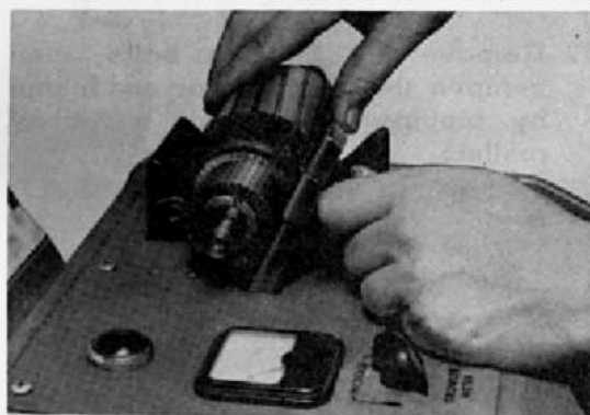
Fig.7-25 Testing Armature for Open Circuit W2745
