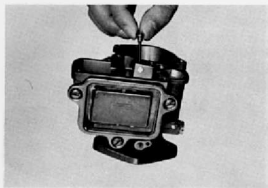
Fig.4-16 Main Air Bleeder Removal V0559
