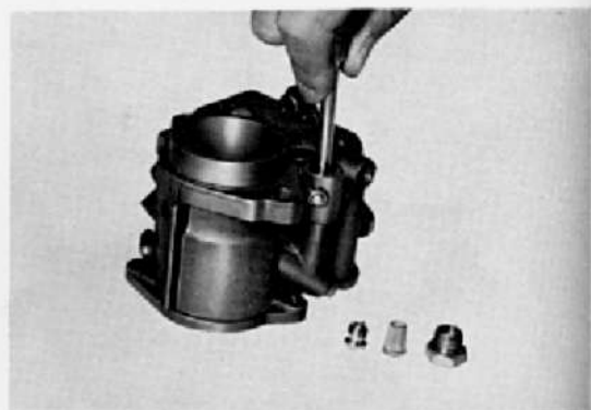
Fig.4-20 Discharge Check Valve Removal V0563
