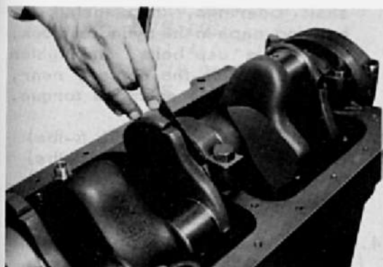
Fig.2-40 Measuring End Clearance V0551
