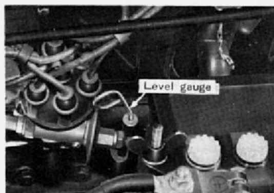
Fig.1-2 Engine Oil Inspection V0547
