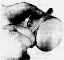
Fig. 3-26 Measuring Groove W5361 Clearance
