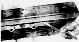
Fig. 3-8 Measuring Points V4347 of Cylinder Head
