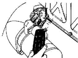
Fig 2-6 Ignition Timing Inspection X4919
