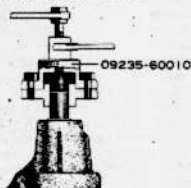
Fig. 7-4 Pulley Seat Removal X5049
