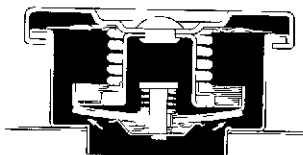
Fig 7-8 Pressure Relief C1110
