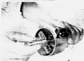
Fig. 8-49 Removing Distributor Cam W0866
