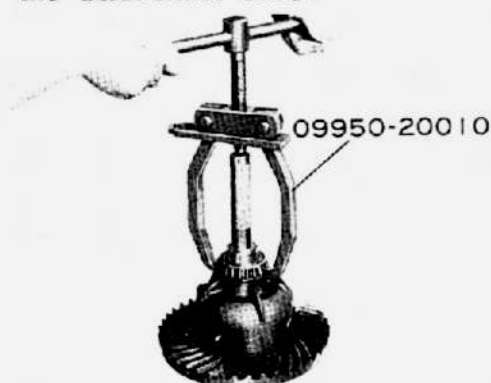
Fig.4-20 Removing Side V5093 Bearing
