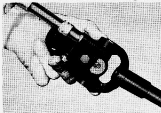
Fig.6-25 Tightening U-bolt V5127 Nut
