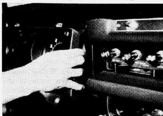
Fig.11-2 Removing Com- B1171 bination Meter & Speedometer
