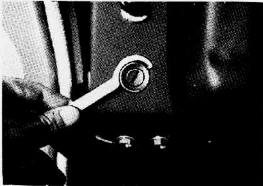
Fig.12-11 Ignition Switch B1181 Removal
