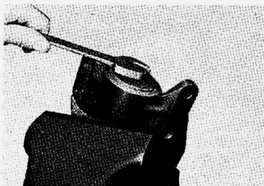
Fig. 6-43 Removing Center V5134 Arm Shaft Nut
