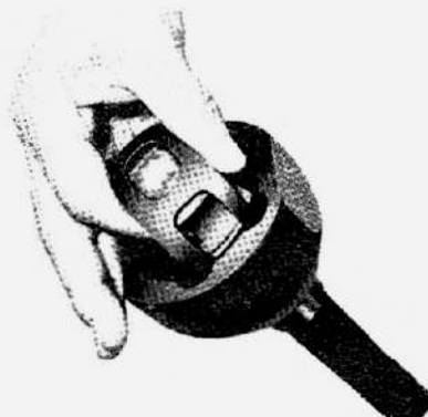
Fig. 5-34 Removing Cage V5112 & Joint Inner Race
