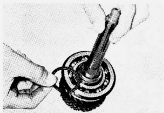
Fig.2-50 Selecting Shaft Snap Ring V5172
