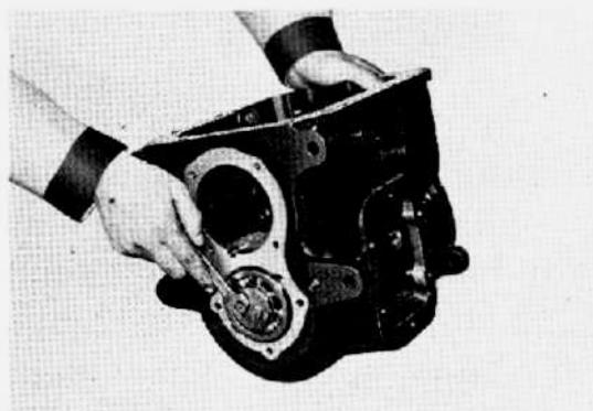
Fig. 2-84 Removing Bearing V5069 Retaining Bolts
